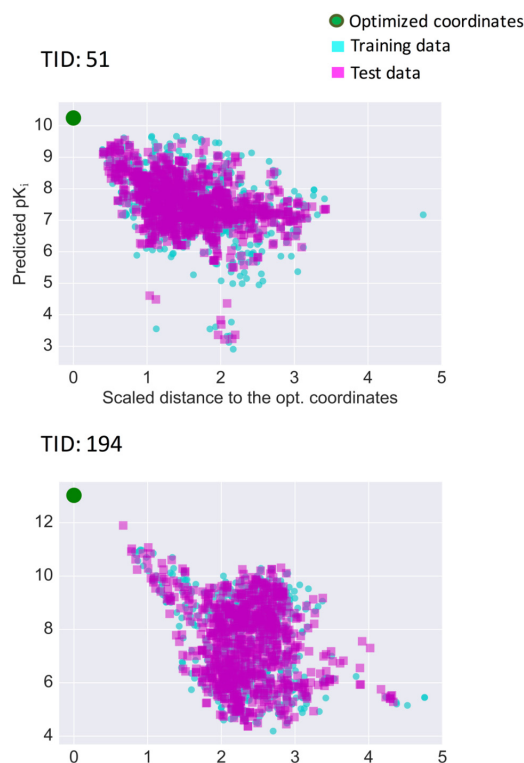
Figure 5. Activity prediction. For two exemplary activity classes, predicted pK_i values are related to the scaled distance of the corresponding compounds to the optimized coordinates. Training data (cyan squares), test data (magenta squares), and optimized coordinates (green circle) are shown.
